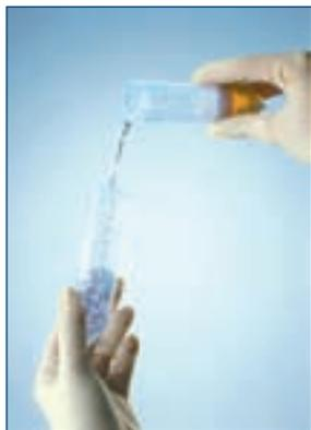
The MaXtract gel forms a safe and stable barrier between the organic solvent and the nucleic acid-containing aqueous phase, enabling simple separation by pouring.
